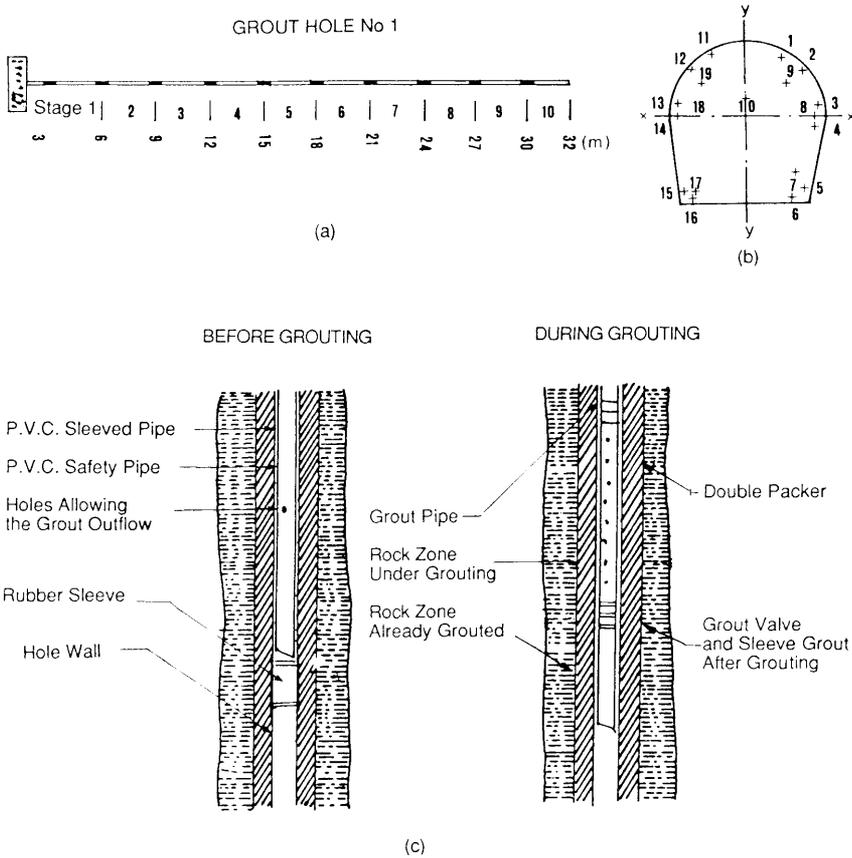
Figure 9. Layout of Grouting Arrangement (a) Details of Multiple Packers in the Boreholes (b) Borehole Layout (c) Details of Grouting.
