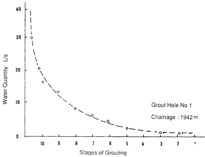
Figure 10. Typical Grouting Effect in Water Quantity Decrease.
