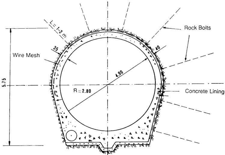
Figure 4. Designed, Finished Profile of Tailrace Tunnel.
