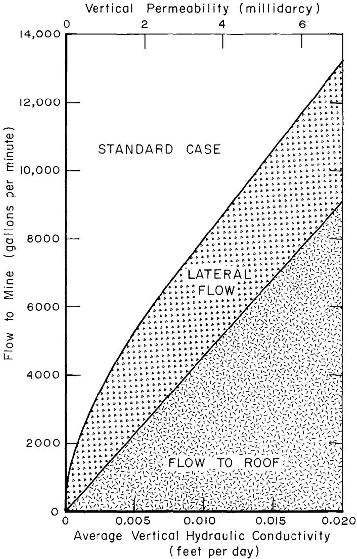
Figure 9 - Relationship Between Inflow and Vertical Hydraulic Conductivity
