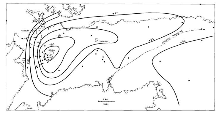
Figure 9 - Regional Piezometric Surface of Basal Aquifers
