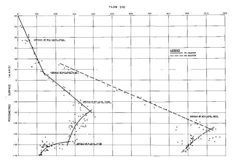
Figure 6 - Relationships Between Piezometric Level and Flow
