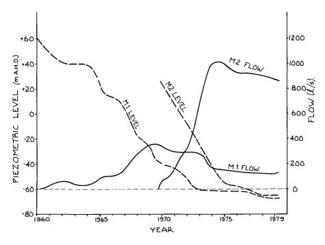
Figure 5 - Piezometric Levels and Flows
