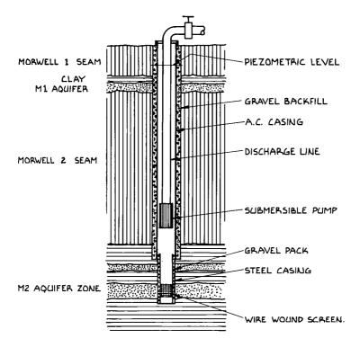
Figure 7 - M2 Aquifer Pumping Bore
