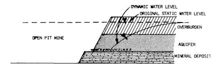
FIGURE 3. DEWATERING BY THE MEANS OF HORIZONTAL DRAINS
