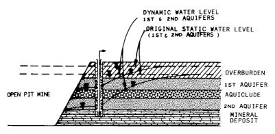
FIGURE 4. DEWATERING BY THE MEANS OF VERTICAL WELLS FROM SURFACE
