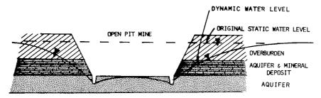
FIGURE 2. DEWATERING BY THE MEANS OF BOTTOM PIT DITCHES
