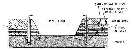
FIGURE 4. DEWATERING BY THE MEANS OF VERTICAL WELLS FROM SURFACE
