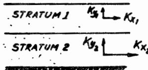
FIG. 4(c). Layered Anisotropic Soil Conditions
