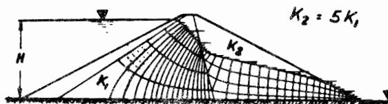
FIG. 4(d). Flow Through Dam Constructed of Two Materials
