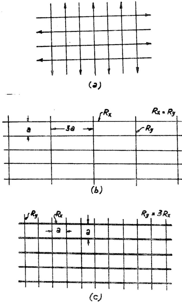
FIG. 2. Two Methods of Modelling Anisotropic Soils
