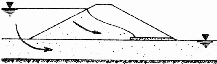
FIG. 1(a). Flow of Water Through Tailings Dam
