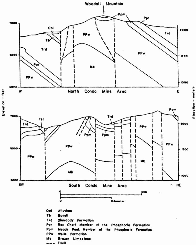
Figure 7. Geologic sections through north and south Conda Mine areas [3]
