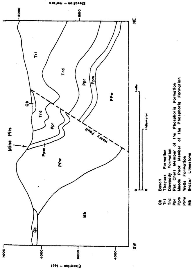
Figure 4. Generalized geologic section through North Henry Mine site [3]
