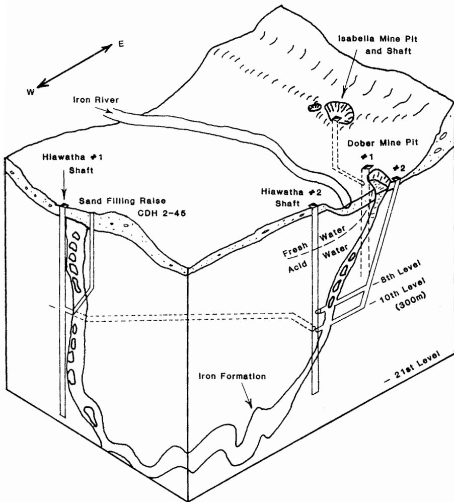
Figure 4. Isometric Sketch of the Dober Mine Complex (Modified from Dutton, 1969).
