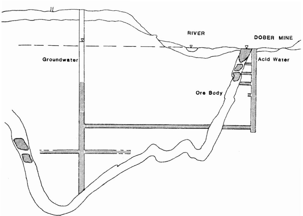
Figure 5. Schematic Representation of Acid Water and Groundwater Distribution in the Dober Mine Complex, Cross-Section Looking Northerly.
