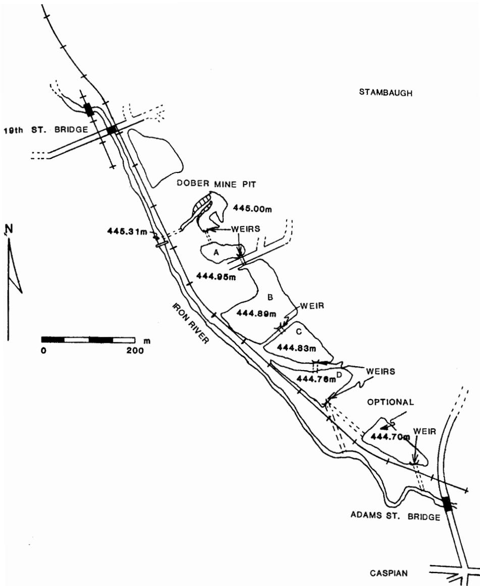
Figure 7. The Proposed Water Diversion/Pond System For Acid Water Treatment at the Dober Mine.
