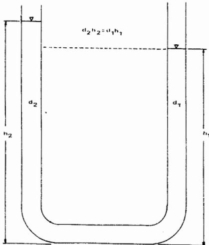
Figure 6. A "U-Tube" Concept to Illustrate Mine Water Elevation Variations as a Function of Water Density.
