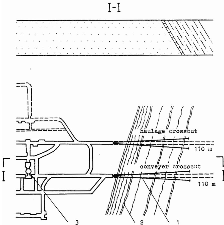
**Fig.1.** Advanced grouting scheme for water bearing strata in driving the 960-m level crosscuts of Nagolchanskaya mine
