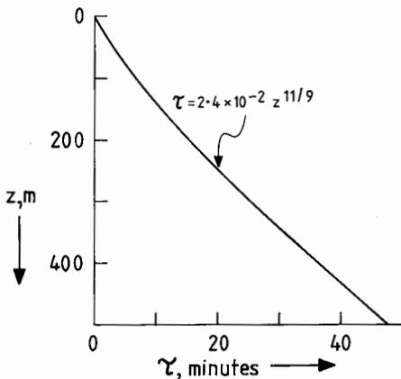
FIGURE 3.  $\tau$  VERSUS  $z$  FOR MAXIMUM PRESSURE-INDUCED FLOW
