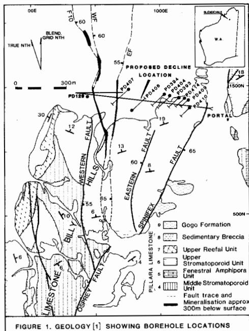
FIGURE 1. GEOLOGY [1] SHOWING BOREHOLE LOCATIONS
