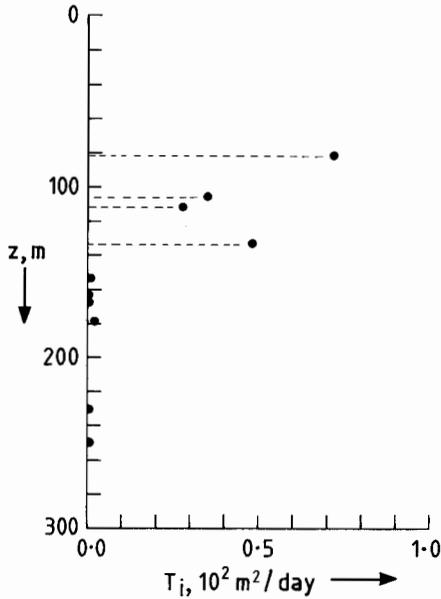
FIGURE 2. TRANSMISSIVITY OF EQUIVALENT APERTURES, PD129
