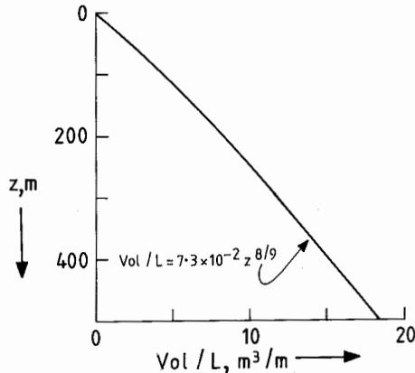
FIGURE 4.  $\text{Vol}/L$  VERSUS  $z$  FROM A VERTICAL FRACTURE DURING  $\tau$
