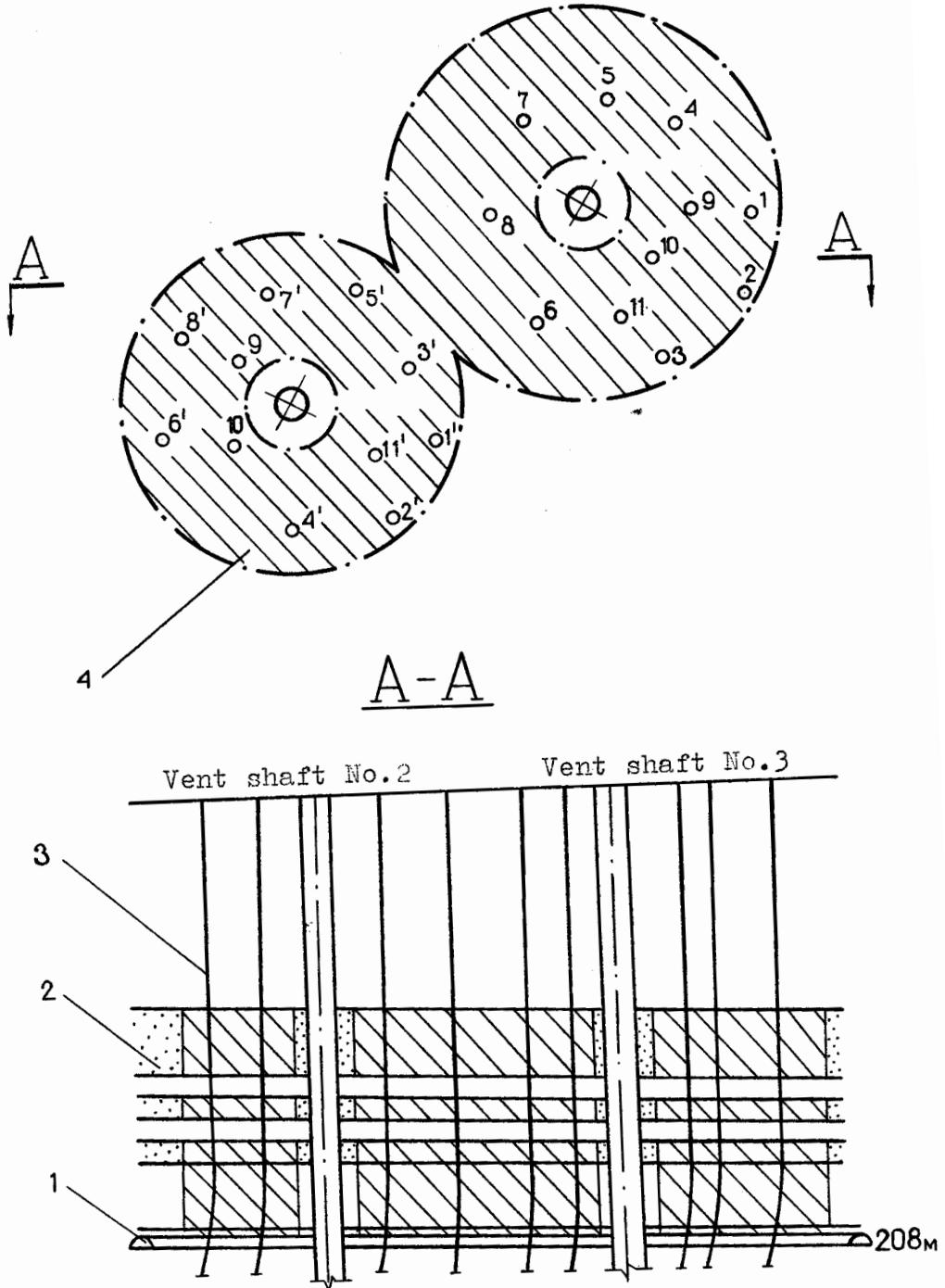
Fig. 1 Grouting procedure for abandoned workings around mine shafts of the Yuzhnaya Mine
