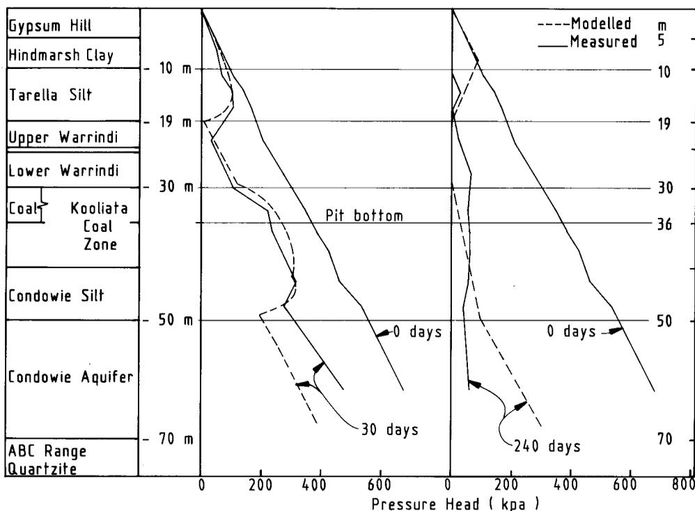
Figure 4. Actual versus predicted drawdown at centre of pit
