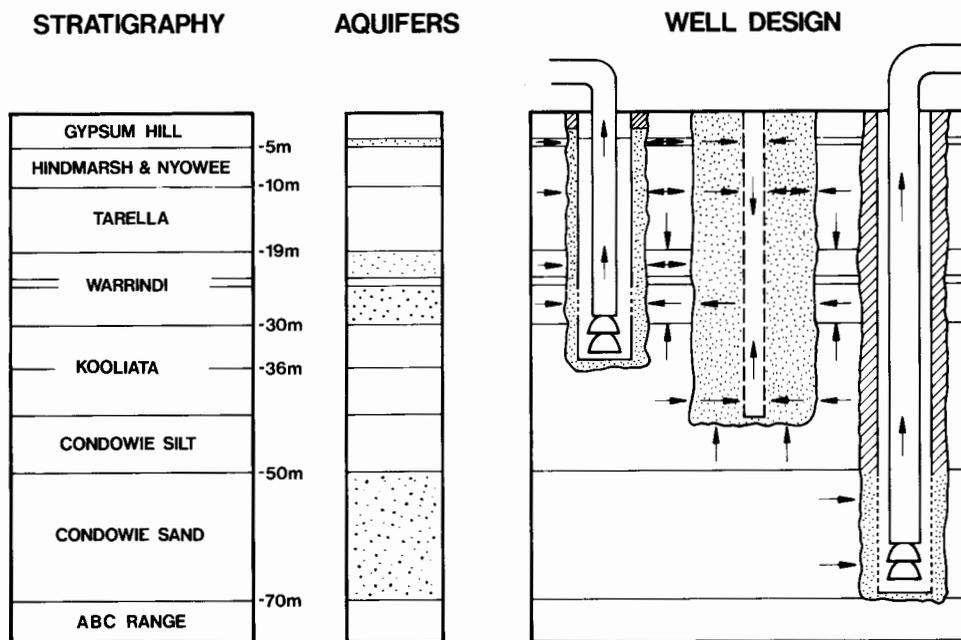
Figure 2. Design and interaction of water wells
