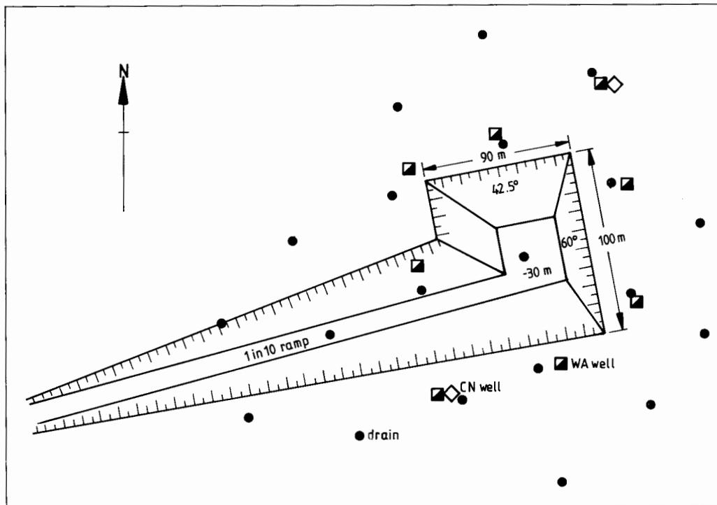
Figure 1. Pit design and well location plan
