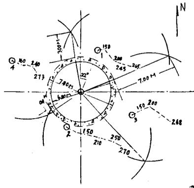
Fig.1 Geometry of grout hole pattern and deviation plan
