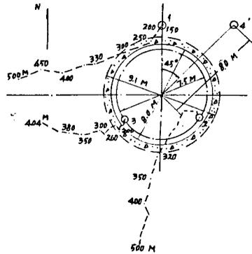
Fig. 2 Grout hole pattern and deviation plan of a colliery in Shangdong province
