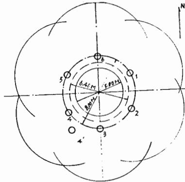
Fig. 3 Grout hole pattern and design of an ideal closed curtain wall for central air shaft in Shandong
