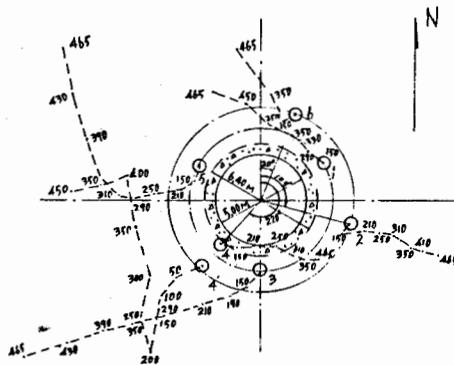
Fig. 4. Actual grout hole pattern in operation and deviation plan of central air shaft of a colliery in Shandong
