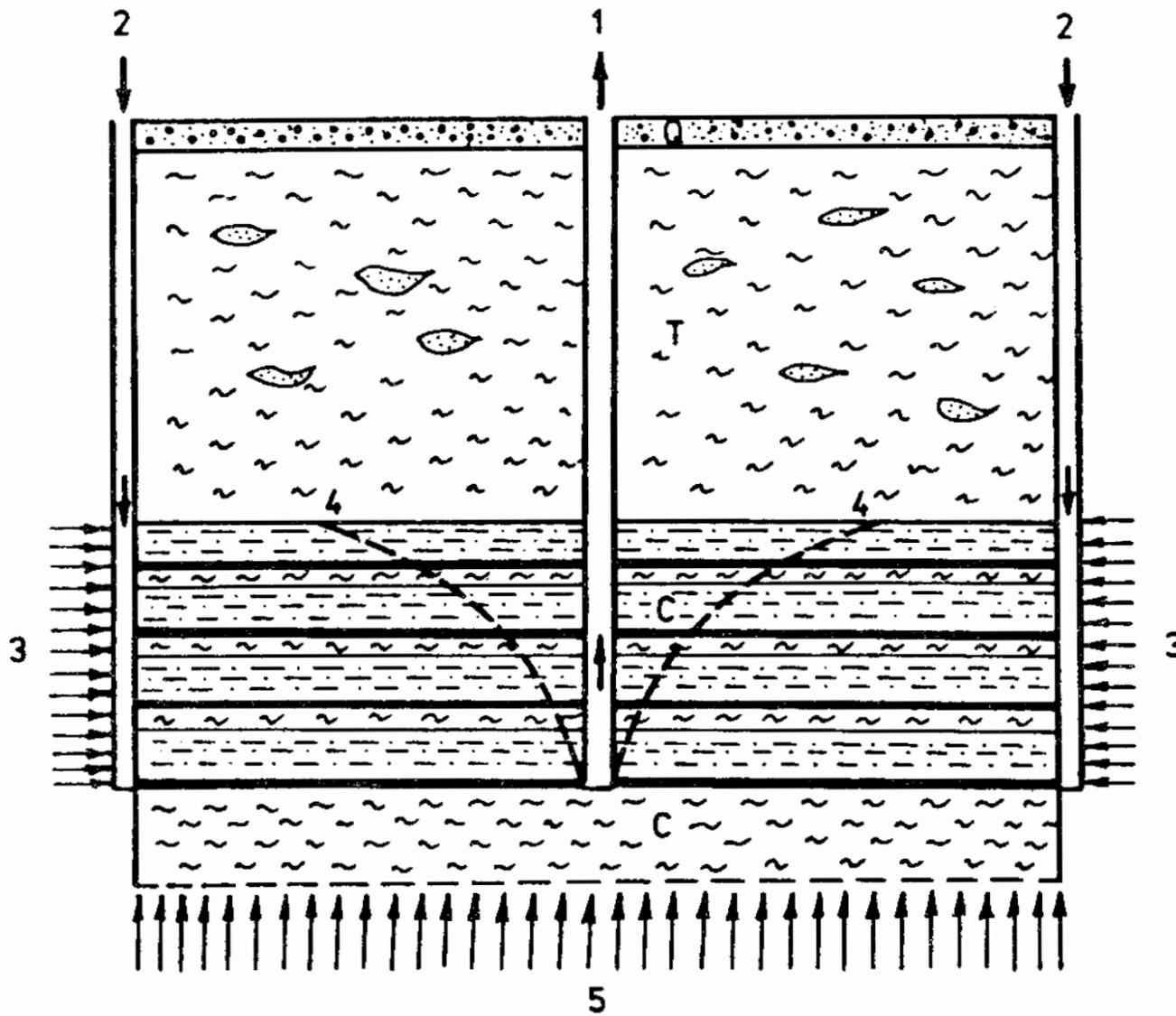
Legend: Q-Quaternary, T-Tertiary + Triassic, C-Carboniferous, 1-exploitation well, 2-reinjection well, 3-water inflow. 4-cone of drainage, 5-heat flux
