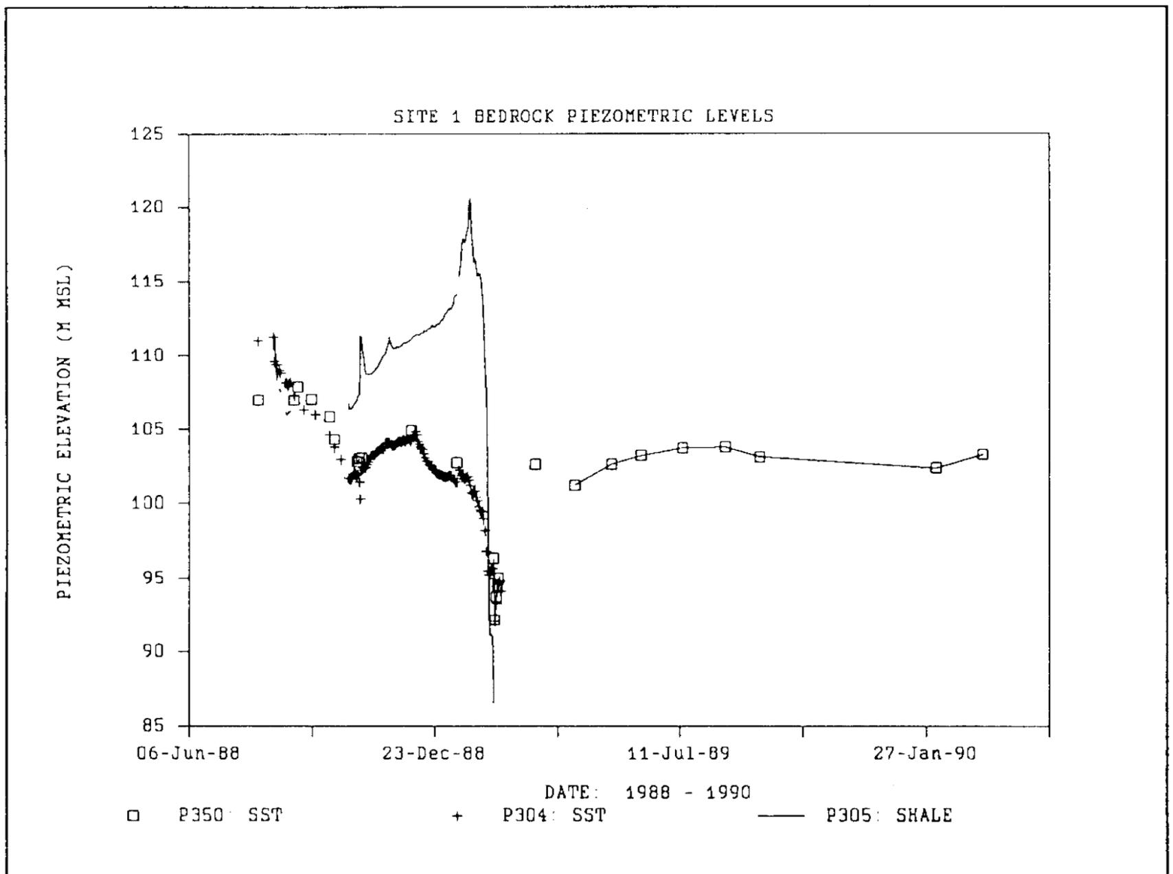
Figure 2. Site 1 Bedrock Potentiometric Levels
