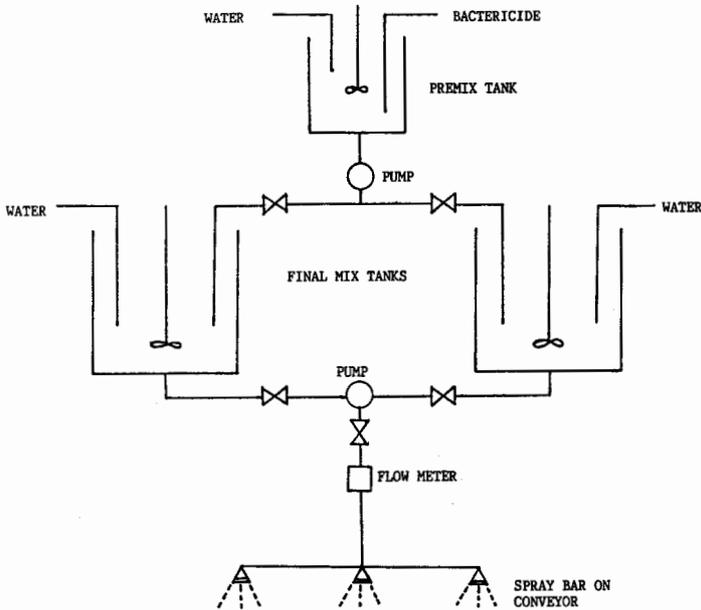
Figure 2. Automatic spray system for continuous treatment of coal reject as it exits the plant on a conveyor system.
