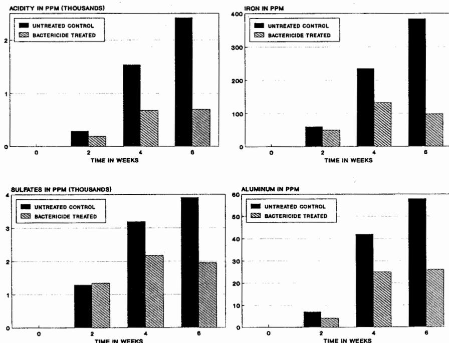
Figure 1. Results from column leach tests on coal company coal reject with and without (control) bactericide treatment to show control over acidity, sulfates, iron, and aluminum with bactericides.
