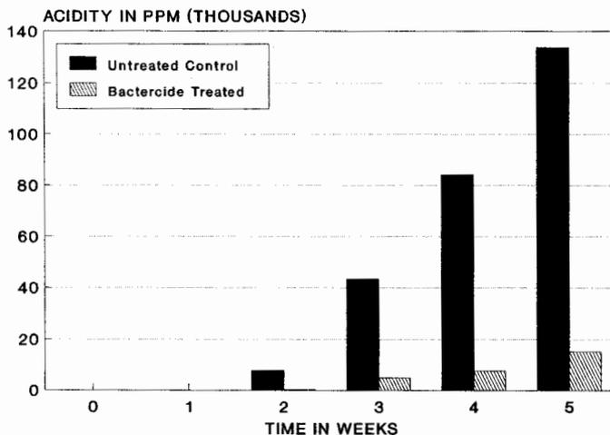
Figure 6. Results from column leach tests on power plant coal reject with and without (control) bactericide treatment showing control of acid generation.
