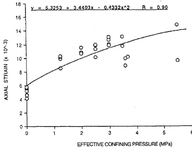
FIGURE 2 - Variation of axial strain at failure with effective confining pressure.
