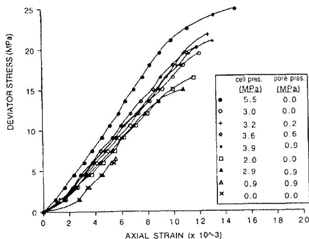
FIGURE 1 - Typical average stress-strain curves for drained test specimens with the same effective confining pressure.
