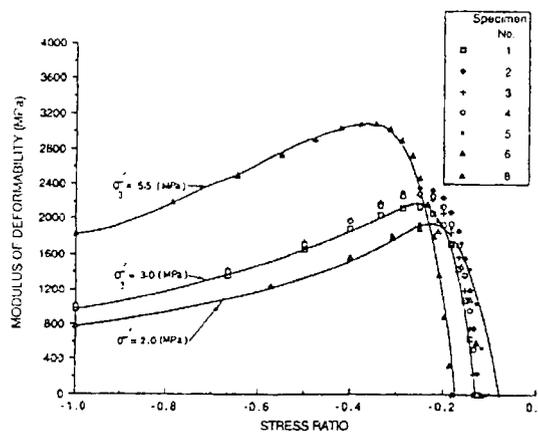
FIGURE 7 - Variation of modulus of deformability with stress ratio,  $k = \sigma_3'/\sigma_1'$ .
