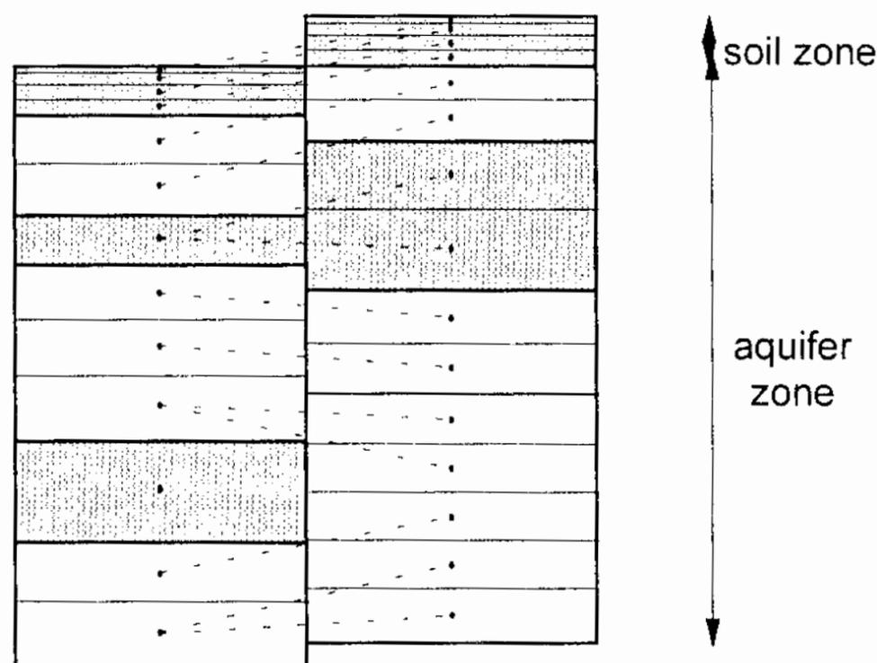
Figure 3b: VSS Computational Cell Definitions and Interconnections
