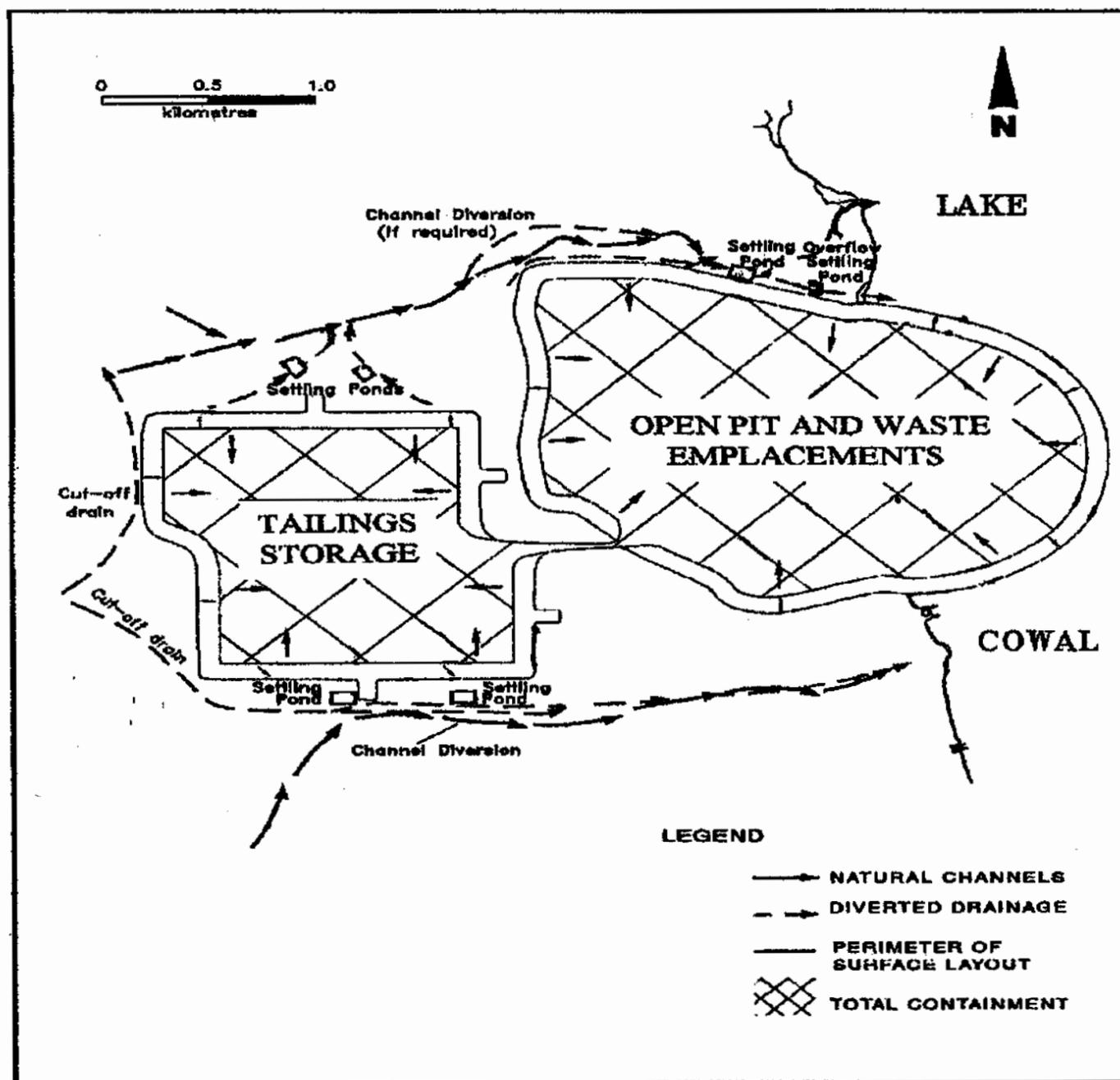
Figure 2: Mine site layout, drainage and water management plan (after NSR, 1996)
