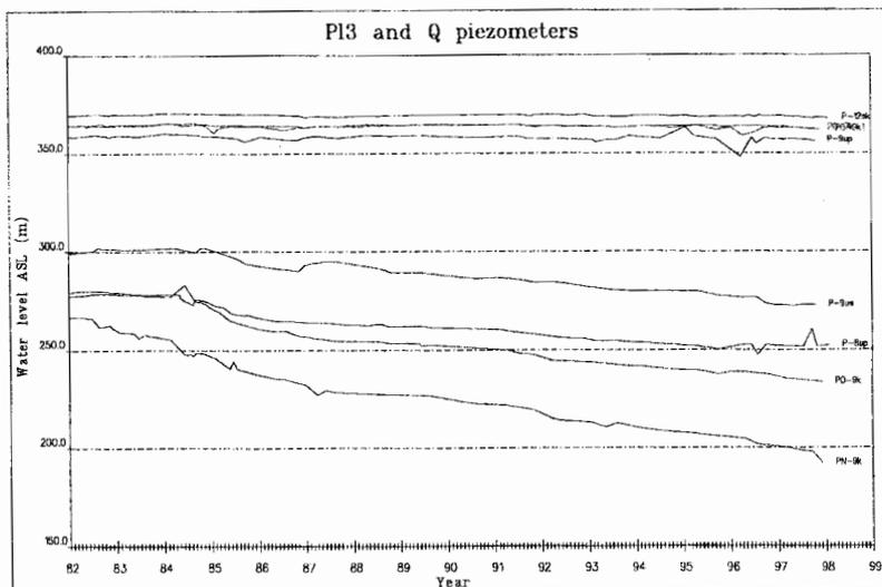
Fig. 6: Examples of water table oscillation on piezometers that belong to the  $P_3$  and Q (quaternary) aquifer complex
