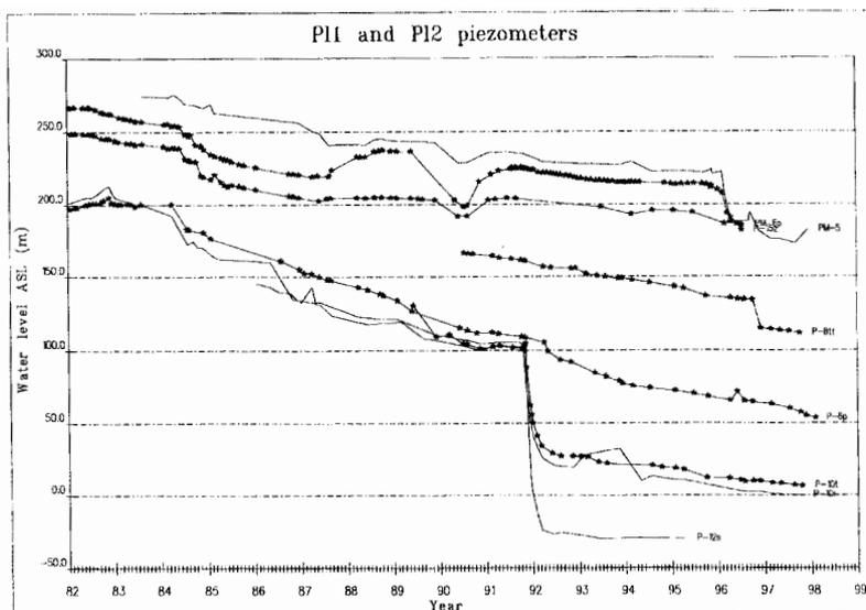
Fig. 5 Examples of water table oscillation on piezometers that belong to the  $PI_1$  and  $PI_2$  aquifer complex.
