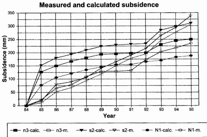
Fig. 7: Calculated and measured subsidence for three chosen measuring points
