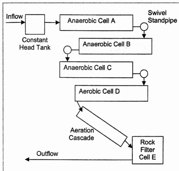
Figure 2. Schematic diagram of constructed wetland system (Not to scale).
