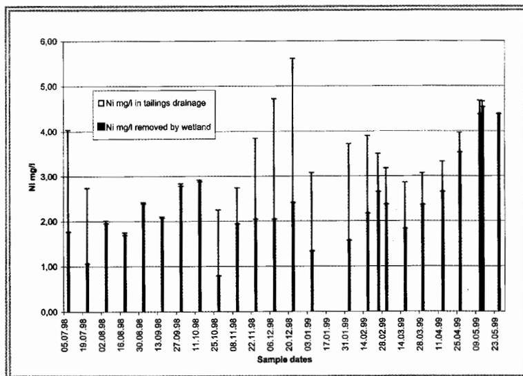
Figure 3. Concentrations of nickel in the tailing drainage and removed in the wetland.
