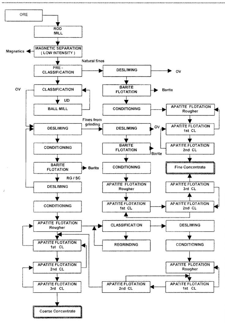
Figure 1. Original flowsheet of the concentration plant.
