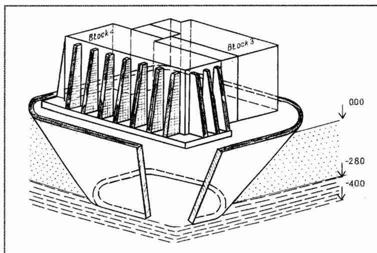
Figure 2. Encasement of the block 3 &amp; 4 of the Chernobyl NPP.
