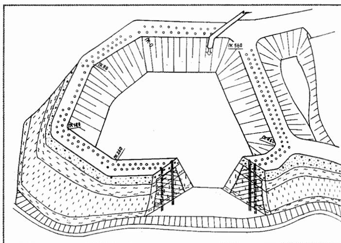
Figure 1. Arrangement of grout holes around tailing pond No. 1 of the Nicopol Ferroalloy Factory
