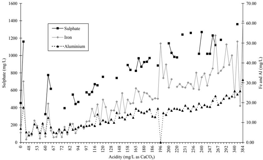
**Fig. 3.** Relationship between increasing acidity concentration and increases in concentration of Fe, Al and  $\text{SO}_4$ , for tip leachate at Deerplay.
