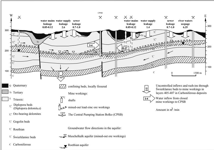
Fig. 2. Hydrogeological cross-section.
