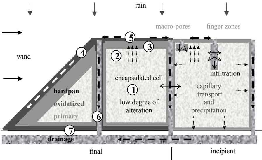
**Fig. 3.** Section through a slag heap showing different diagenetic stages. Zones of drainage, infiltration and capillary transport are shown in conjunction to the evolution of an oxidation rim and subsequent hardpan formation and encapsulation of cells (1-7; see text).
