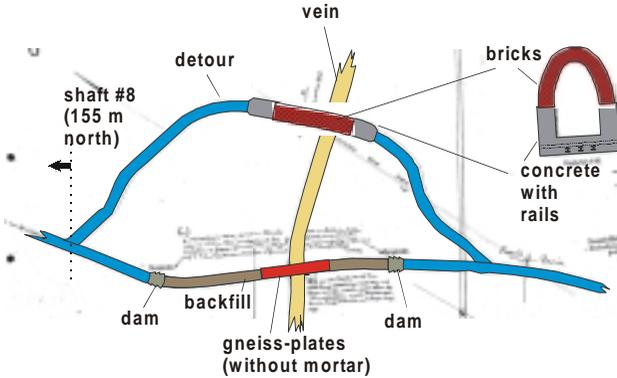
Figure 2: Scheme of the adit with bypass driven in 1897
