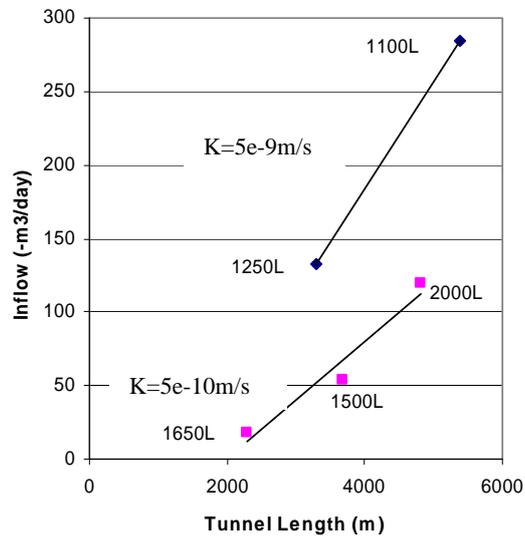
**Fig. 2.** Graph showing relationship between cumulative 1D tunnel length and inflow for two bedrock conductivity zones
