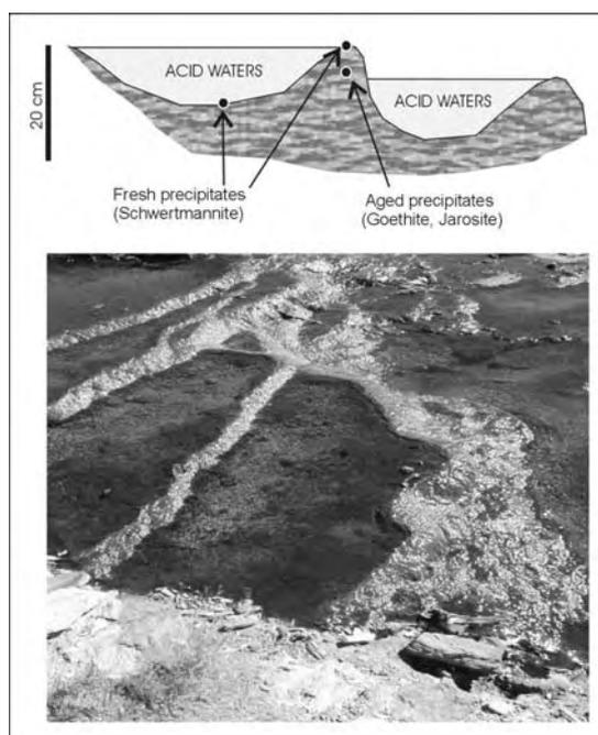
**Figure 2: Typical view of one of the sampling points and position of the points for sampling precipitates in the terraces of the Monte Romero abandoned mine.**
