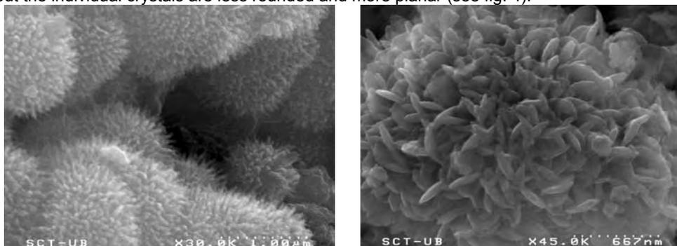
**Figure 4: Scanning Electron Microscopy images of the precipitates at the beginning (left) and at the end (right) of the laboratory experiment on schwertmannite durability.**
