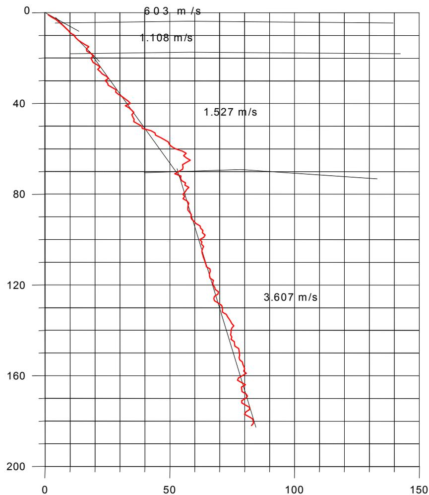
**Fig 7: Transit Time diagram and Velocities for the PZ2**
