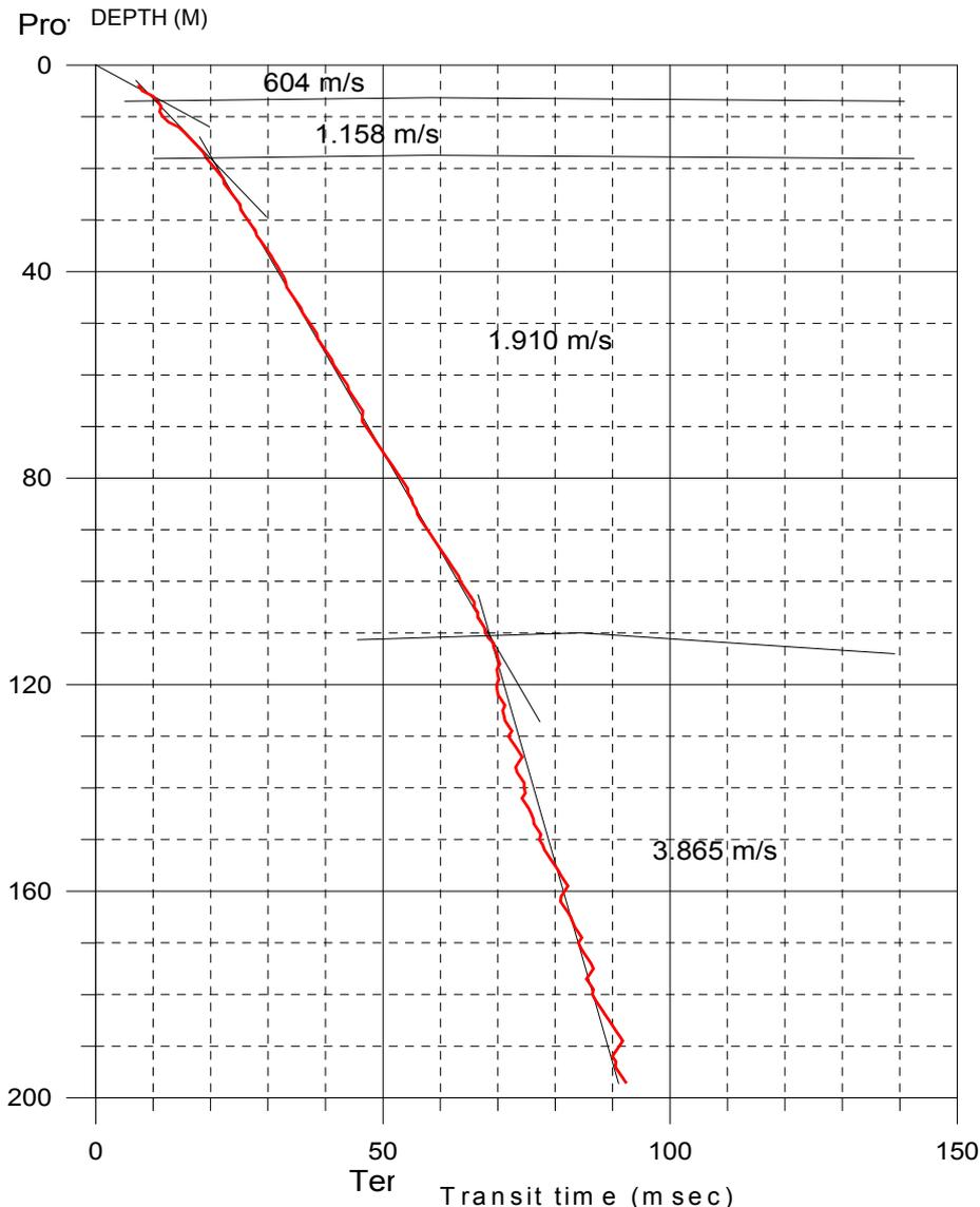
**Fig 6: Transit Time diagram and velocities for the PZ1**
