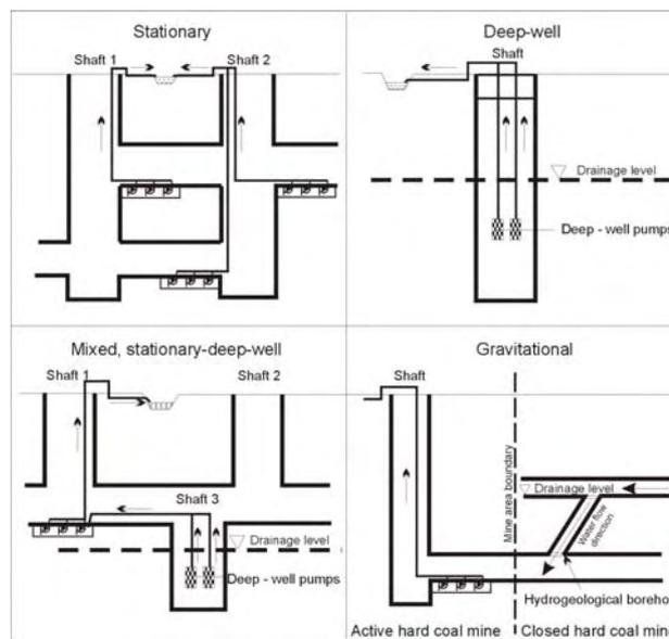
Figure 3: The drainage systems in the closed hard coal mines
