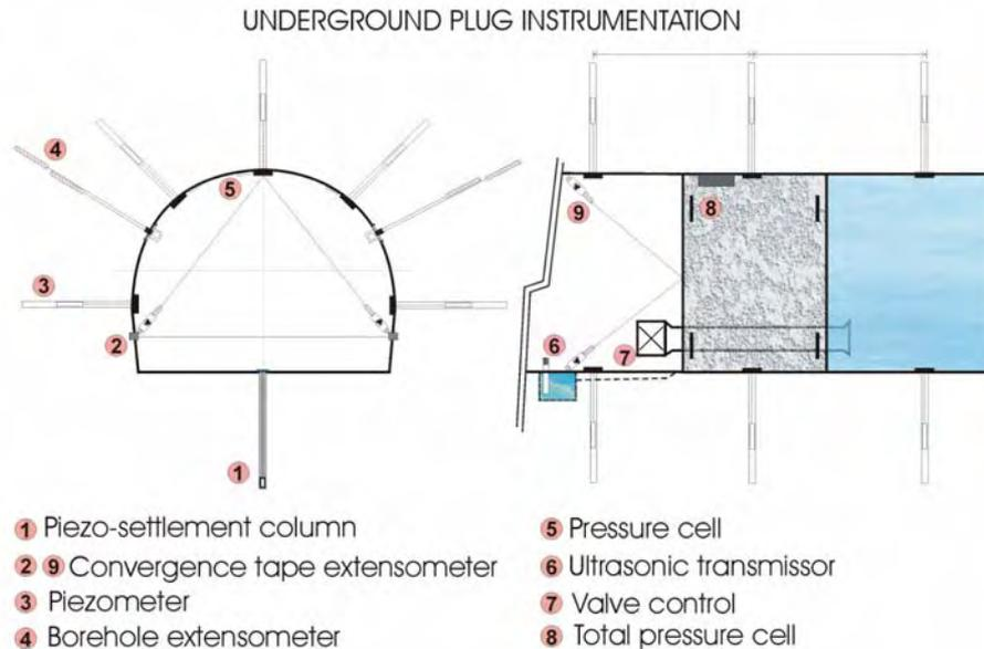
**Figure 15: General scheme of instrumentation for an underground plug monitoring**
