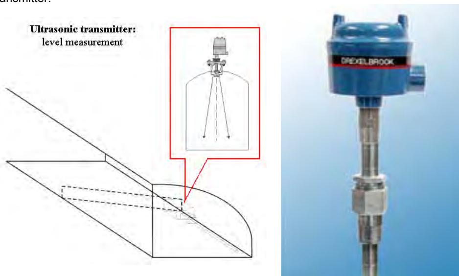
**Figure 14: Flow measurement principle. Ultrasonic transmitter.**
