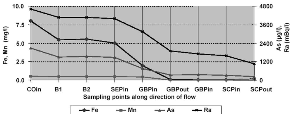
Figure 4: Contaminant concentration at sampling points along direction of flow through wetland
