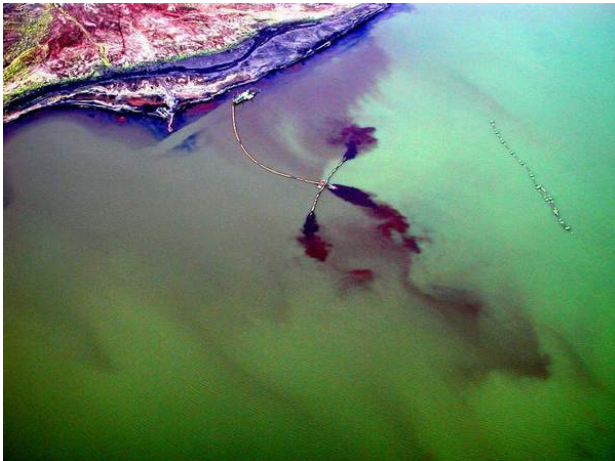
Figure 3. Re-suspension of fly ashes from the lake bottom without the use of CO 2 (courtesy of eta AG engineering Cottbus).
