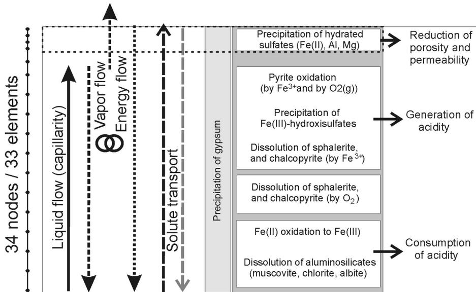
**Figure 1. Main thermohydraulic and geochemical processes included in the model.**
