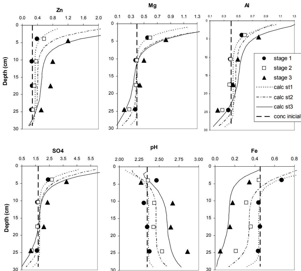
**Figure 3. Evolution of concentration ( $\text{mol}\cdot\text{kg}^{-1}$ ) and pH of porewater from the columns. Comparison with calculated values.**
