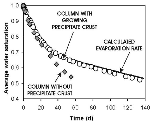
**Figure 2. Evolution of the evaporation rate of two representative columns. Comparison with calculations.**
