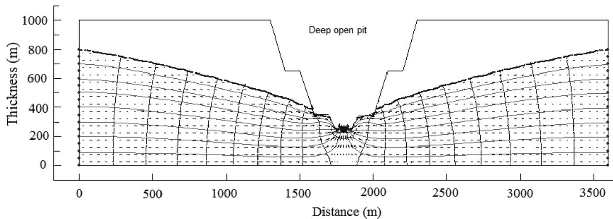
Figure 4. The results of two-dimensional modelling for a deep open pit mine in an unconfined aquifer.
