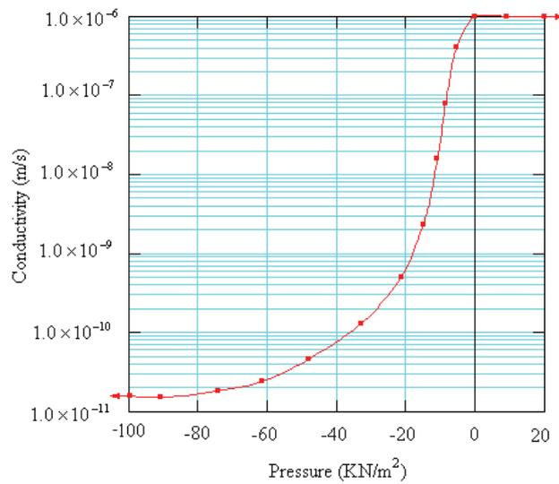
Figure 3. Hydraulic conductivity as a function of pore water pressure.
