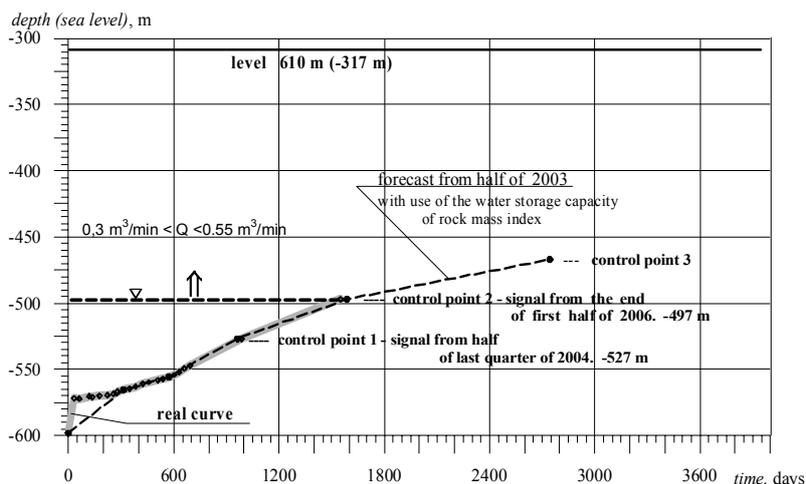
**Figure 4. Changes of groundwater level in mine workings in the abandoned "1-Maja" mine up to the second half of 2006.**
