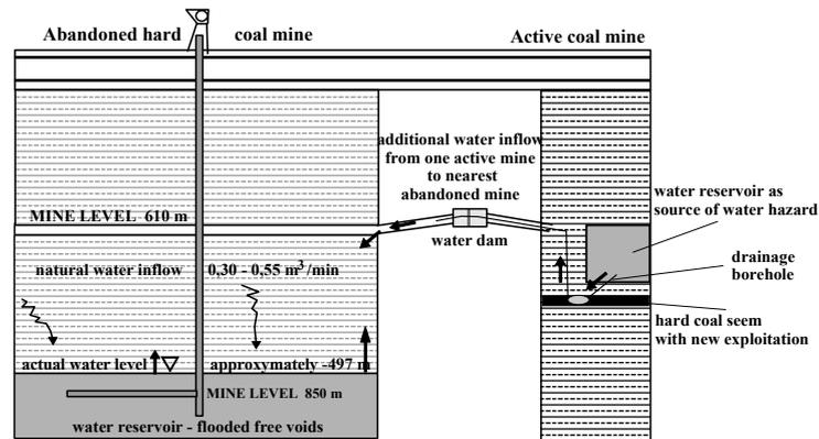
Figure 5. Scheme of using the free voids in abandoned mine by the active coal mine.
