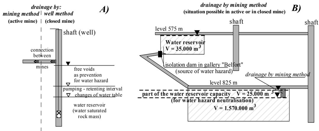
**Figure 3. Models of use of free voids as a protection against water hazard (after Bukowski et al., 2006):**
