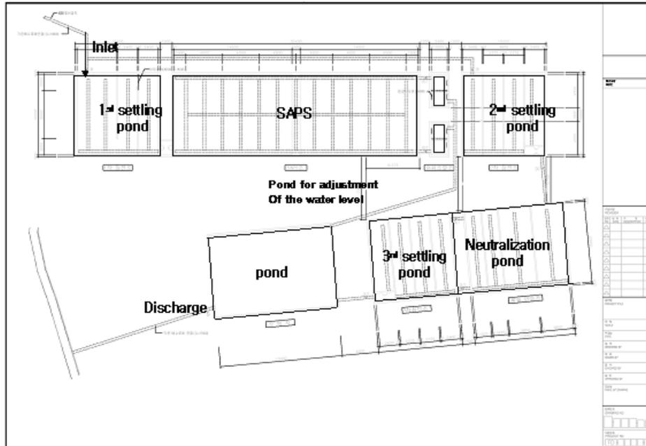
Figure 1. Plan view of existing passive treatment system.
