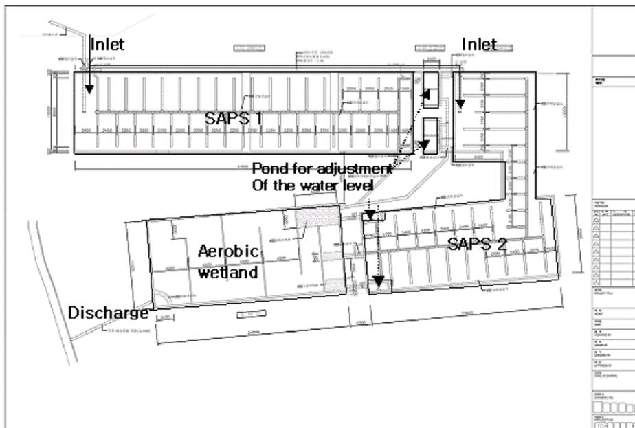
Figure 2. Plan view of renovated passive treatment system.
