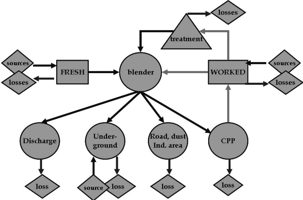
**Figure 1. System diagram of a simplified coupled salt and water balance model for a mine site (Moran and Moore, 2005).**
