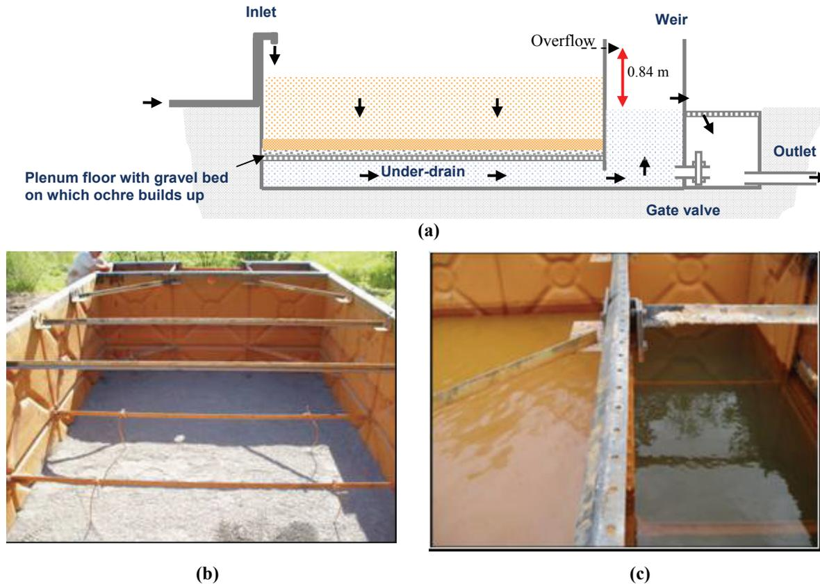
**Figure 1. The VFR. (a) Schematic; (b) After installation of new gravel bed; (c) Ocherous downflow (left), clean upflow (right).**
