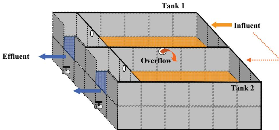
**Figure 2. Schematic of two VFRs running in parallel.**
