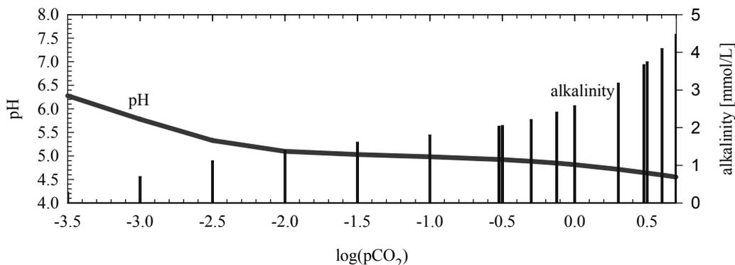
**Figure 3. Reaction lake water with  $\text{CO}_2$  at 10 °C after addition of 2.5 mmol  $\text{Fe}^0$ ; simulated at equilibrium pH after precipitation of siderite.**
