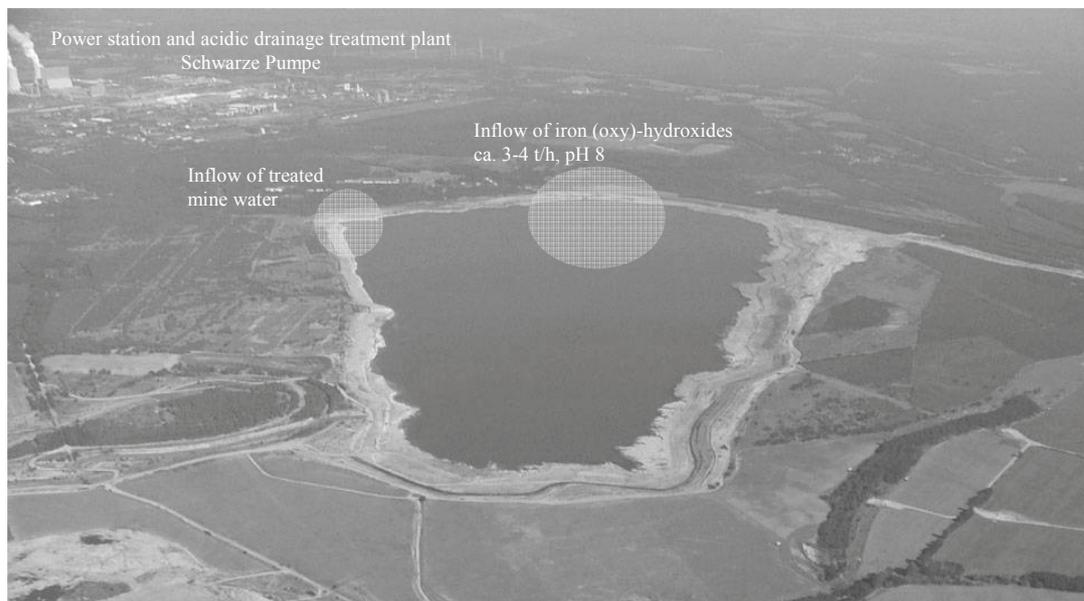
**Figure 1.** Aerial view of the Spreetal-Nordost mining lake (September 23<sup>rd</sup> 2005 at 1000 m height eta-AG, orientation to East). The acid mine treatment plant Schwarze Pumpe is located in the upper left corner.
