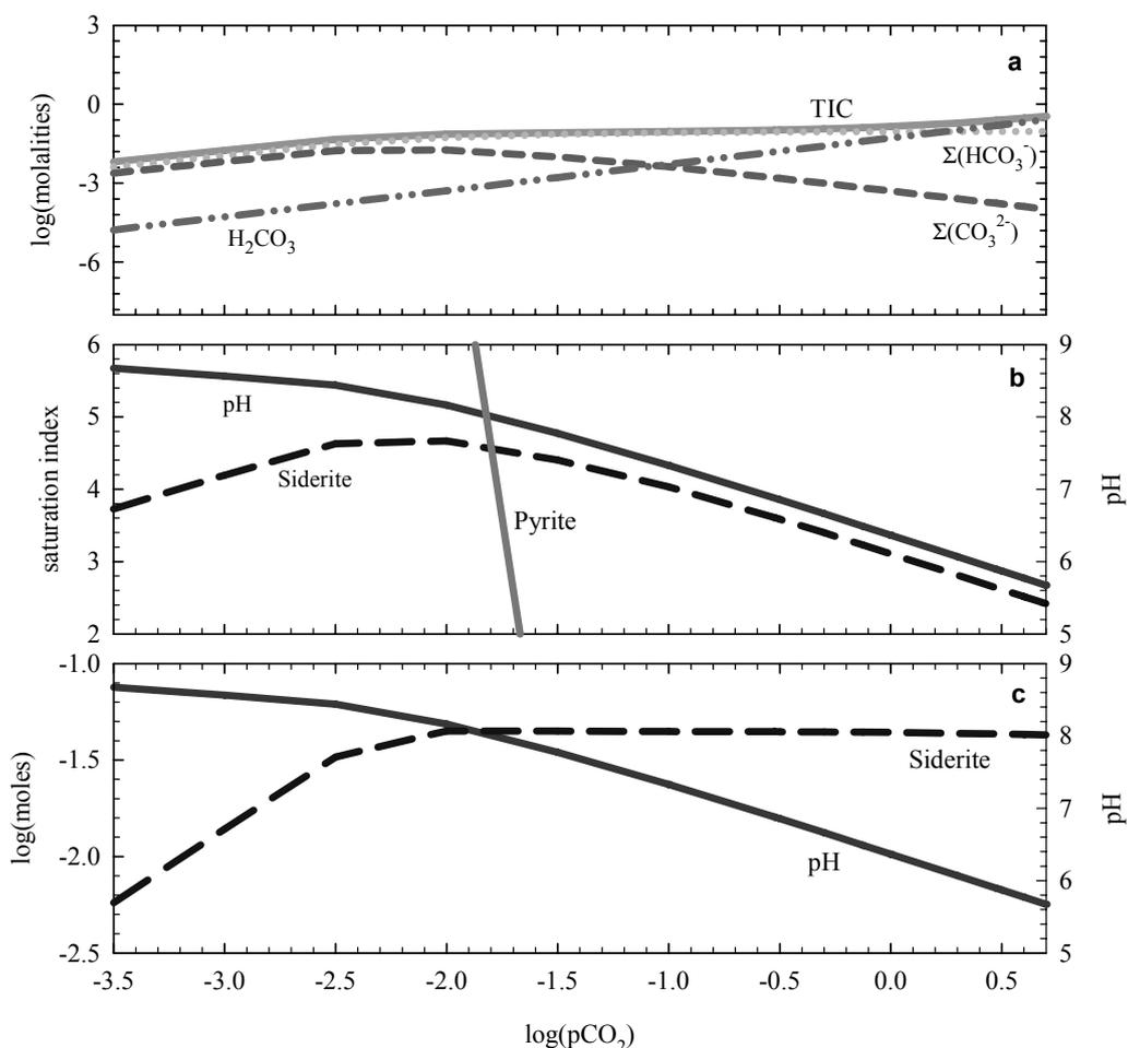
Figure 2. Species distribution for the reaction of lake water with  $\text{CO}_2$  at 10 °C after addition of 2.5 mmol  $\text{Fe}^0$ ; simulated at equilibrium.
