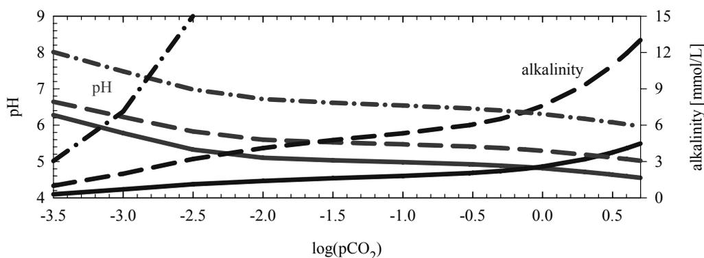
**Figure 5. Comparison of alkalinity and pH after precipitation of siderite at different saturation indices; solid lines:  $SI_{\text{siderite}} = 0$ , dashed lines:  $SI_{\text{siderite}} = 1$ ; addition of 2.5 mmol  $\text{Fe}^0$ .**
