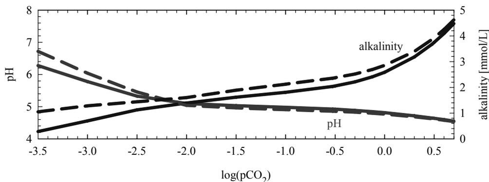
**Figure 4. Comparison of alkalinity, pH and siderite precipitation after reaction of lake water, iron (oxy)-hydroxides and  $\text{CO}_2$ ; solid lines: addition of 2.5 mmol  $\text{Fe}^0$ , dashed lines: addition of 10 mmol  $\text{Fe}^0$ .**
