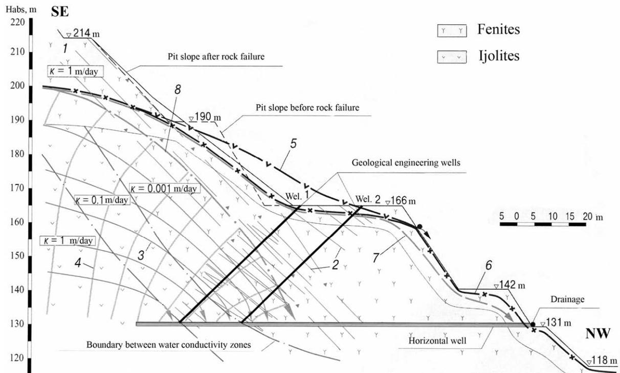
**Figure 3** Scheme of seepage with horizontal well working:
