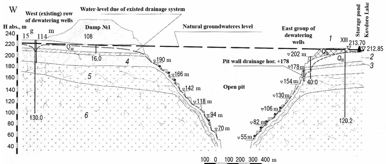
**Figure 2** Hydro-geological section along line 1 — 1 (see Figure 1): 1 — embankment; 2 — alluvial sediments; 3 — disintegration zone; 4 — interconnected strong fissuring zone; 5 — interconnected weak fissuring zone; 6 — uninterconnected weak fissuring zone.
