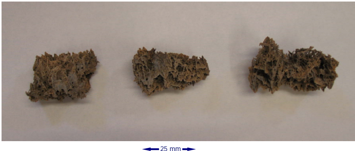
Figure 3. Calcite Lattice Growth in Carlton Tunnel Sediment Ponds
