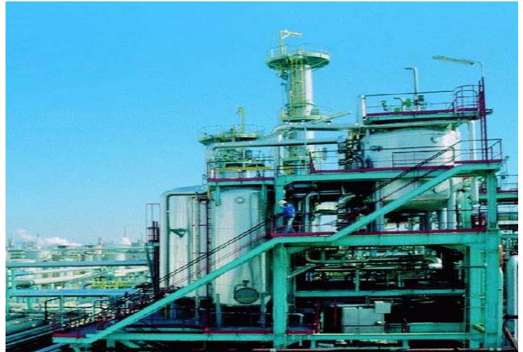
Picture 4. Crystalactor for nickel and aluminium recovery from spent catalysts
