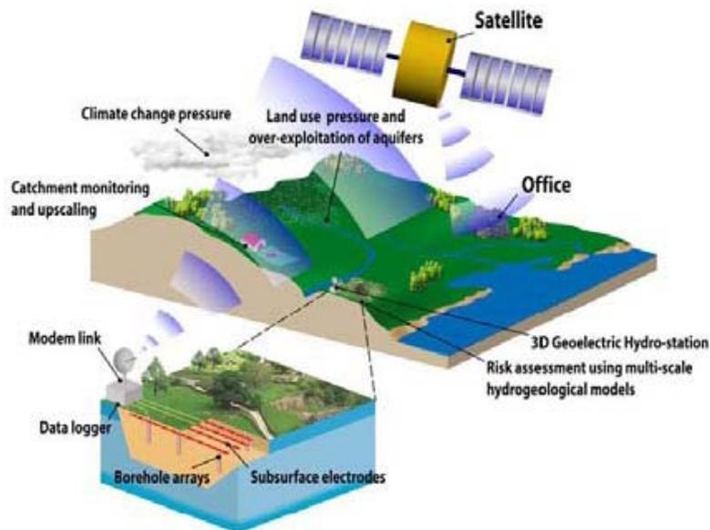
Fig 1. Schematic ALERT concept showing buried ERT
