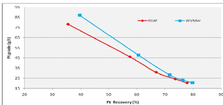
Figure 6. Effects of Rustenburg Treated Sewage Effluent (RSW) and Waterval Merensky Process Water on Platinum Flotation at Rustenburg
