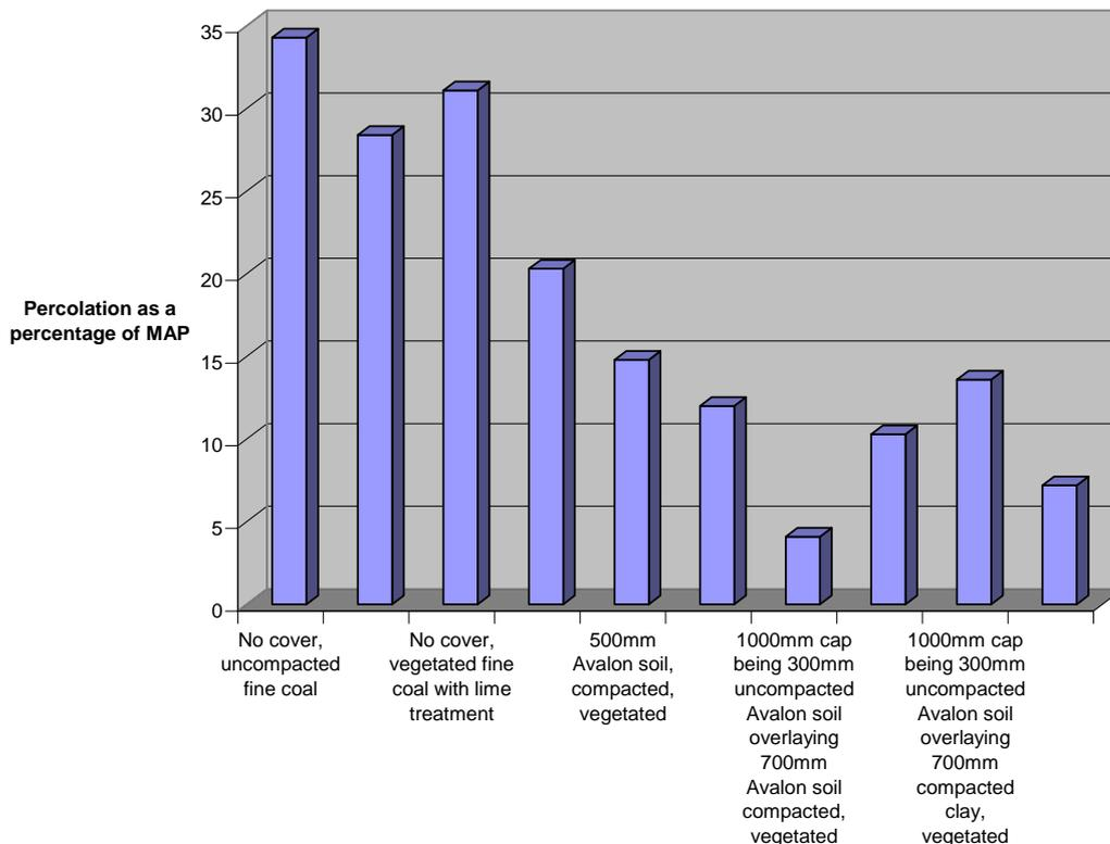
Figure 5. Reduction in infiltration related to the thickness of capping layers (Bezuidenhout,2004)
