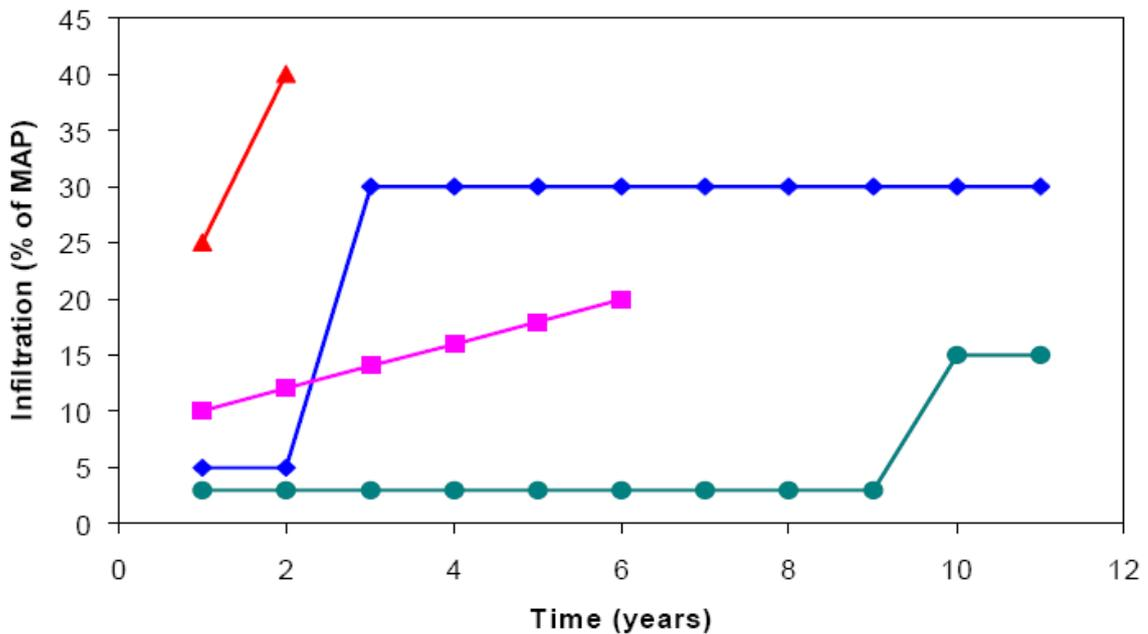
Figure 2. Long term monitoring data indicating the change in infiltration rates with time for four sites (Rykaart et al)
