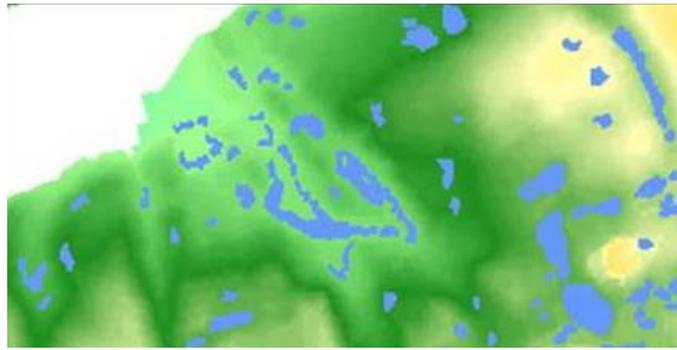
Figure 3. Plan showing a detailed survey of a rehabilitated area showing numerous localised non-freedraining areas
