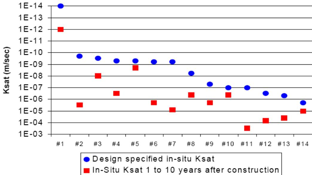
Figure 1. Comparison of designed and measured hydraulic conductivities (Rykaart et al)
