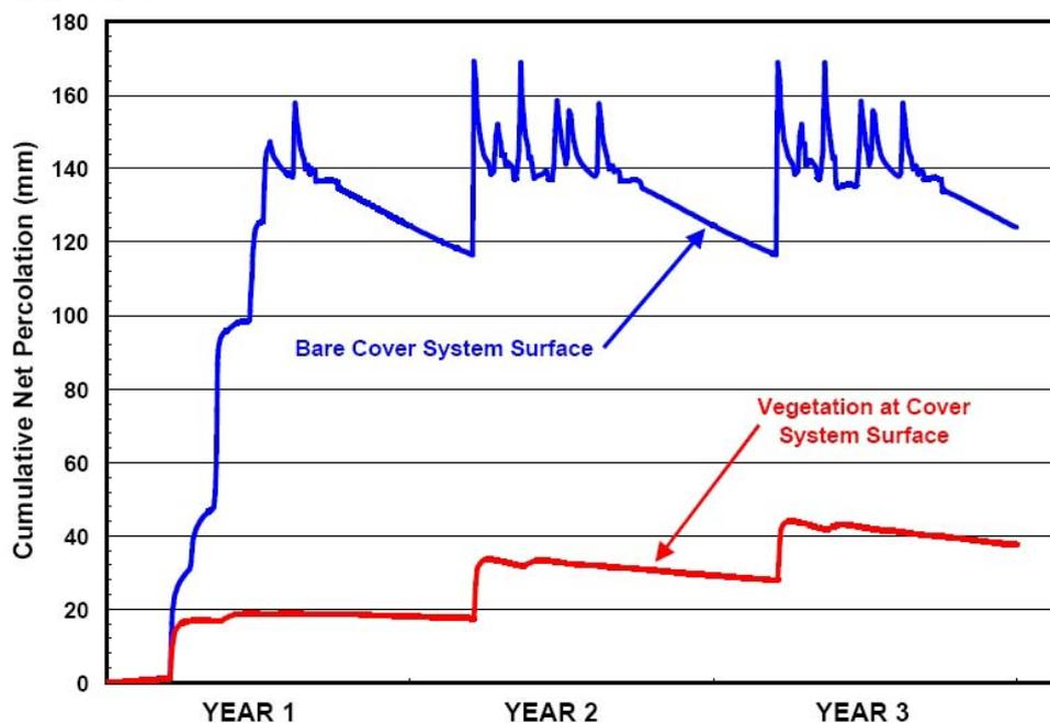
Figure 4. Affect of vegetation on the performance of capping systems as modelled (O'Kane, 2003)
