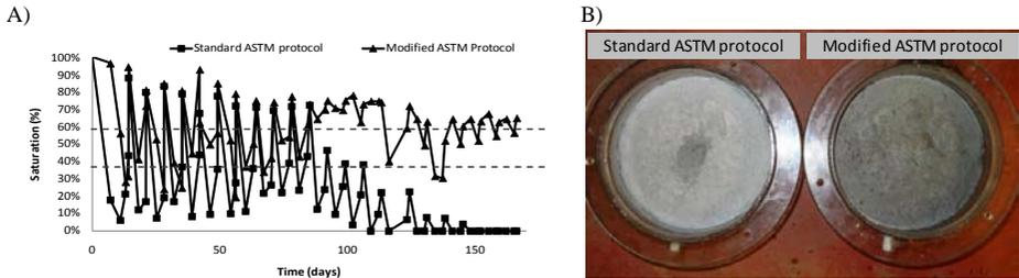
Figure 2 A) Saturation profile in the two humidity cells. The two horizontal lines represent the targeted  $S_r$  values (between 40% and 60%). B) The picture shows that the sample in the standard ASTM protocol was completely dry at the end of the dry period of the cycle compared to the modified protocol where sample remained humid (darker colour is related to the higher water content)
