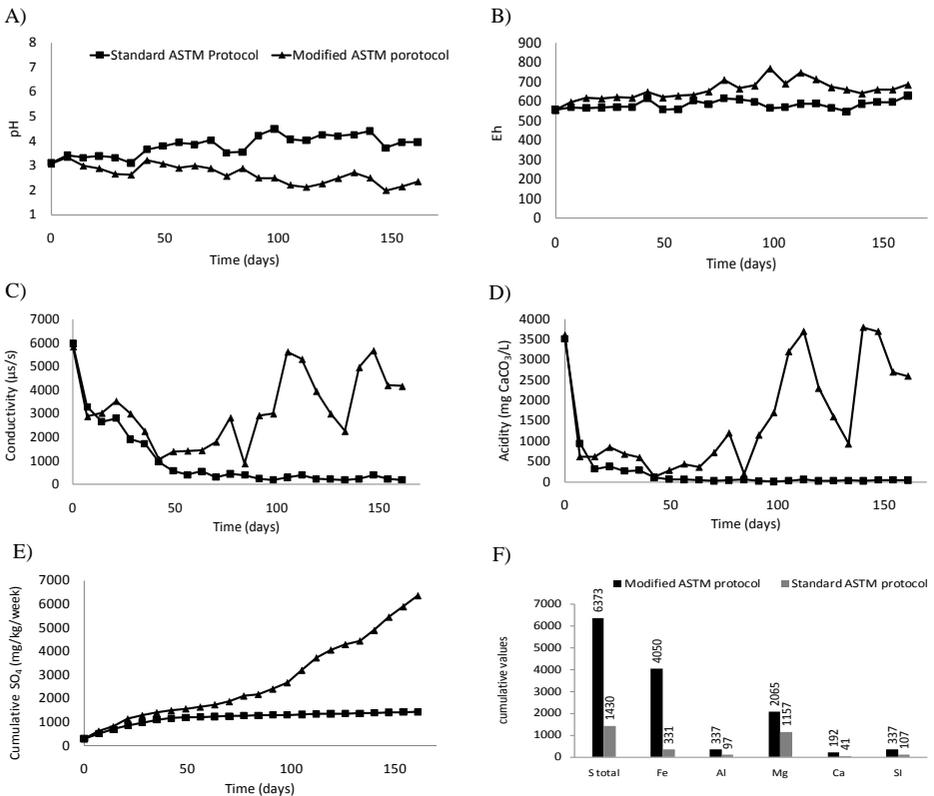
Figure 3 pH, Eh, acidity, conductivity and cumulative sulphate, iron, release after 160 days of kinetic test
