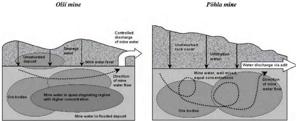
Figure 2 Schematic of water flow in the flooded mines of Olšů and Pöhla
