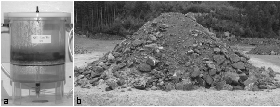
Figure 1 View of a humidity cell (a) and a field test pad (b) installed at the Tio mine site
