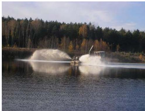
**Figure 1** Spreading boat in action: A slurry of  $\text{CaCO}_3$  and lake water is prepared on the boat and distributed up to 25 meters to each side of the boat. The boat distributes up to 250 tons  $\text{CaCO}_3$  per day
